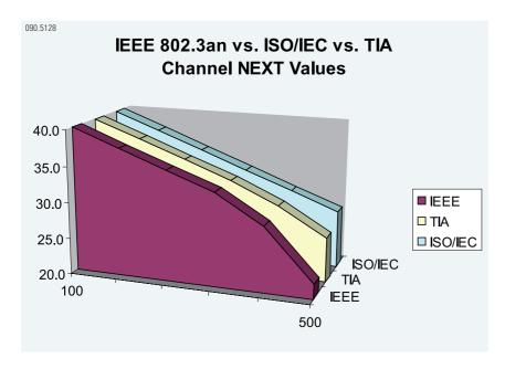
NEXT, the crosstalk at the near end of the channel, is a critical parameter for 10 GbE transmissions. The figure shows the required NEXT values (in dB) over the given frequency (in kHz). Where IEEE bends and EIA/TIA becomes soft, ISO/IEC remains totally consistent, as consistent as Real10 from R&M.
