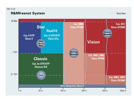
High-performance data networks require fully developed cabling systems such as R&Mfreenet with its Real10 copper range and its Vision fiber optic range for 10 GbE.
